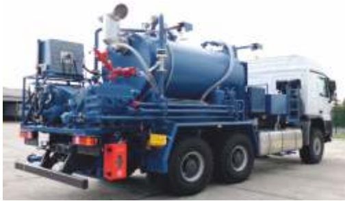
Hot Oil Pumping Unit
